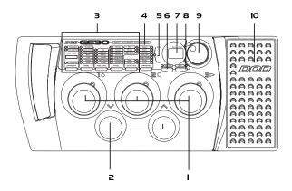
Program Footswitches - These switches provide access to the GS30 user presets. They are also used to bypass the GS30, access the Tuner, and perform various functions for the Learn-A-Lick feature.
